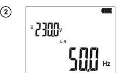
Read the measurement result: voltage in the auxiliary display field, frequency in the main field.
